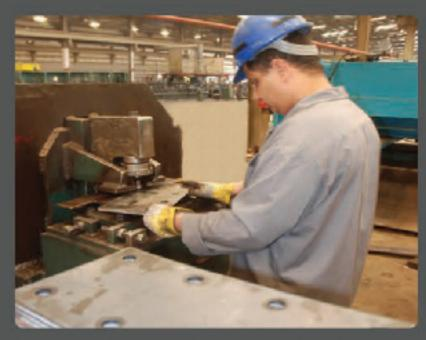
Steel base plates (or columns base plates) are used in the construction of steel frames, such as hangars. These can be produced and delivered with standard holes or plain, depending on customer needs
