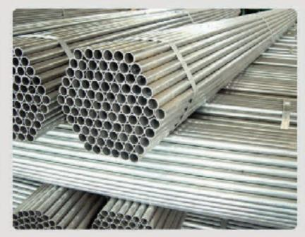
Al Usaimi Co. are committed to provide our customers ideal solutions to tackle the corrosion and rusting problems inherent in all steel products. Galvanizing is a process in which the metal is immersed into molten zinc to form a protective layer which covers steel surface completely, metallurgically sealing it to protect it from corrosive actions of its environment.
